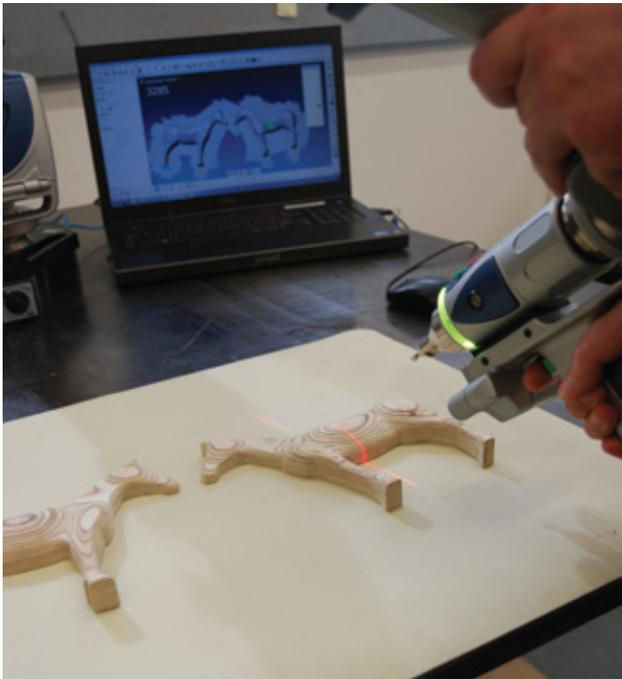
In the photographs above you can see the polygon mesh appearing whilst the toy horse profile is being scanned.
