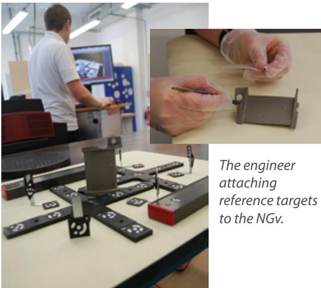
*The engineer attaching reference targets to the NGV.*
