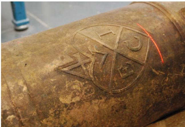
The photograph above shows the cannon with a visible laser line from the 3d scanner.
