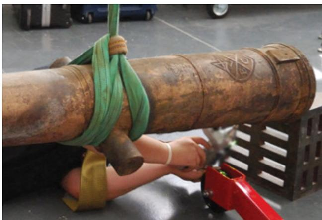
The cannon on a crane being 3d scanned.
